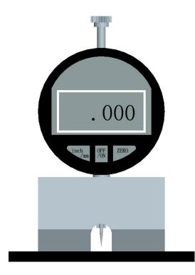
1. Attach the indicator into the hole in the base and lock it with the wrench.
